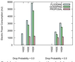
Fig. 6. Total electric power consumption with randomly located nodes.
