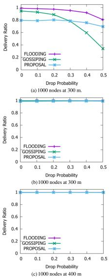
Fig. 4. Information delivery ratio with 1000 randomly located nodes.
