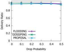
Fig. 5. Information delivery ratio with 1500 randomly located nodes.
